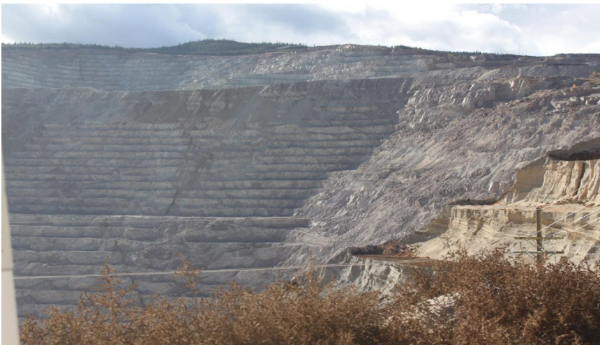
Figure 2. Valley Copper open pit with minor obsequent scarps from toppling in central part of the photo
