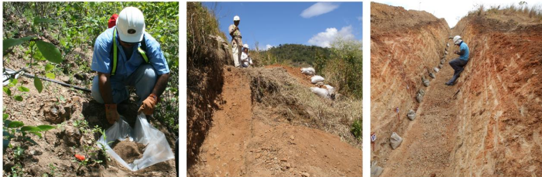
Figure 4. Left: Soil sampling thin soil horizon over weathered felsic volcanic bedrock, and (Centre:) trenches revealing the sandy soil developed over tuff and (Right:) the clayey soil over saprolitic andesite
