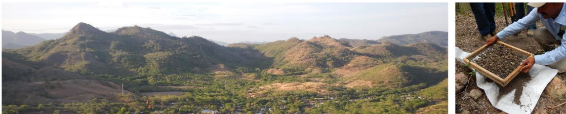
Figure 3. Left: Typical moderate relief landscape in the La India mining district which was covered by a regular grid soil geochemistry survey in 2015-2017. Right: Screening a soil sample at <3 mm mesh to sample the fine fraction in the field
